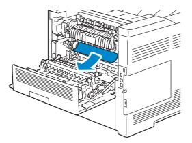
**3** If you cannot see the jammed paper, lift the lever on both sides of the fusing unit.
