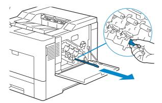
**6** Remove the cleaning pad by pressing the white tabs between your thumb and index finger.
