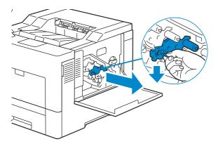
**6** Support the drum cartridge with the other hand from underneath, and then pull it out completely.
