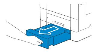
2 Hold the optional 550-sheet feeder with both hands, and remove it from the printer.
