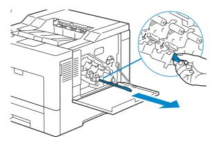
**6** Insert the cleaning rod fully into one of the four holes until it clicks into the interior of the printer as illustrated below, and then pull it out.
