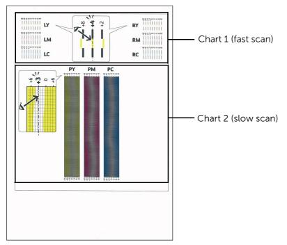
The Chart 1 is used to adjust the color registration for the fast scan direction, which is vertical to paper feed direction. The Chart 2 is used to adjust the color registration for the slow scan direction, which is horizontal to paper feed direction.
