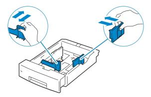
**5** When you load Legal-size paper, extend the tray while pushing the lever located on the front part of the tray.
