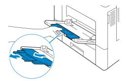
**3** Slide the width guides to the edge of the tray. The width guides should be fully extended.
