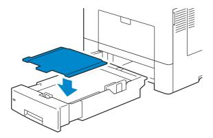
**4** Insert Tray 1 into the printer, and push until it stops.
