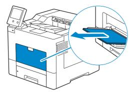
2 Grasp both sides of the bypass tray, and then pull it out of the printer.
