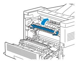
7 Press down the lever on both sides of the fusing unit, and then close the rear cover.
