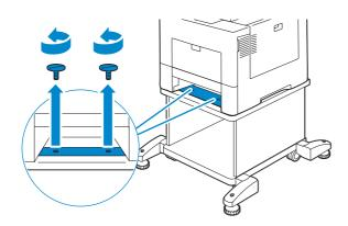
**4** Gently lift the printer off the optional caster cabinet, and place it on a level surface.
