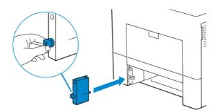
**4** Push and rotate the stopper 90 degrees clockwise until the triangle on the stopper aligns with the one marked on the extender body.
