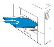
**5** Slide both width guides until they rest lightly against the edge of the print media stack.
