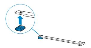
**9** Insert the cleaning rod fully into one of the four holes until it clicks into the interior of the printer as illustrated below, and then pull it out.
