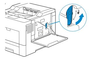
**3** Grasp the handle on the waste toner box and pull it out making sure to hold it upright so that the waste toner does not spill out.
