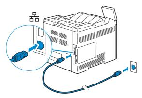
To connect the printer to the network, connect one end of an Ethernet cable into the Ethernet port on the rear of the printer, and the other end to a LAN drop or hub.
