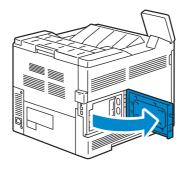
**5** Remove the wireless adapter from the printer by releasing the adapter's hook.
