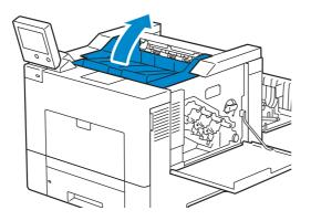
**9** Put your fingers through the loops on both sides of the transfer belt unit, and then pull it out.
