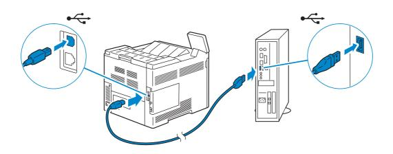
2 Connect the other end of the cable into a USB port of the computer.
