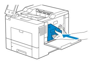
**3** Turn the waste toner box lock lever 90-degrees clockwise to lock the waste toner box.
