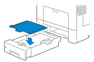
**10** Insert the tray into the printer and push until it stops.
