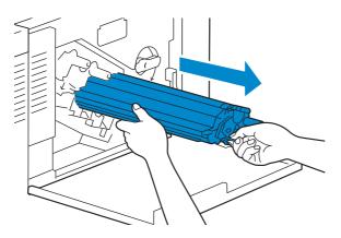
7 Repeat steps 5 and 6 to remove the other three cartridges.
