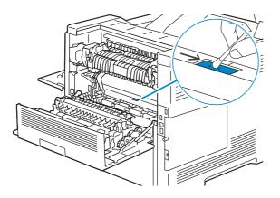
**11** Make sure that the arrow marks on the transfer belt unit and the printer face each other, and then insert the unit into the printer until it clicks.
