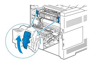
4 Hold and lower the tabs to open the inner part.
